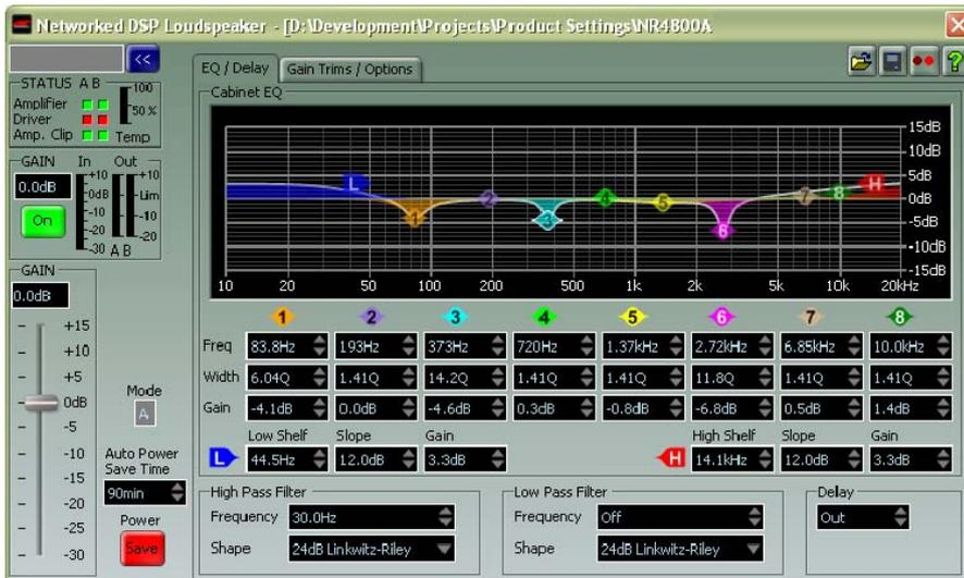
PODWARE provides complete control of Equalisation, Input Filters, Gain, Gain Trim and Delay. PODWARE also provides extensive real-time monitoring of Input & Output Levels, Clip and Limit. Data logging retains Thermal, Protection & Current values for the last 90 Hours of operation.
